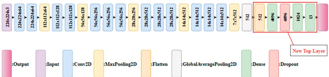
Figure 8. Architecture of customized VGG16 model.
